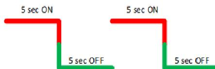
**LNG LEAKAGE ALARM**
