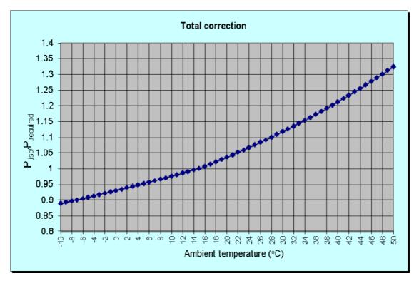
Figure 2: Correction factor of the estimated compression power in ISO conditions in relation with of the ambient temperature at sea level
