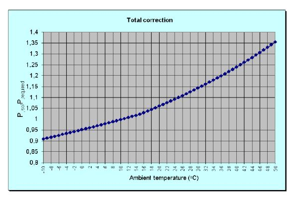
Figure 1: Correction factor of the estimated compression power in ISO conditions in relation with of the ambient temperature at 190m altitude.
